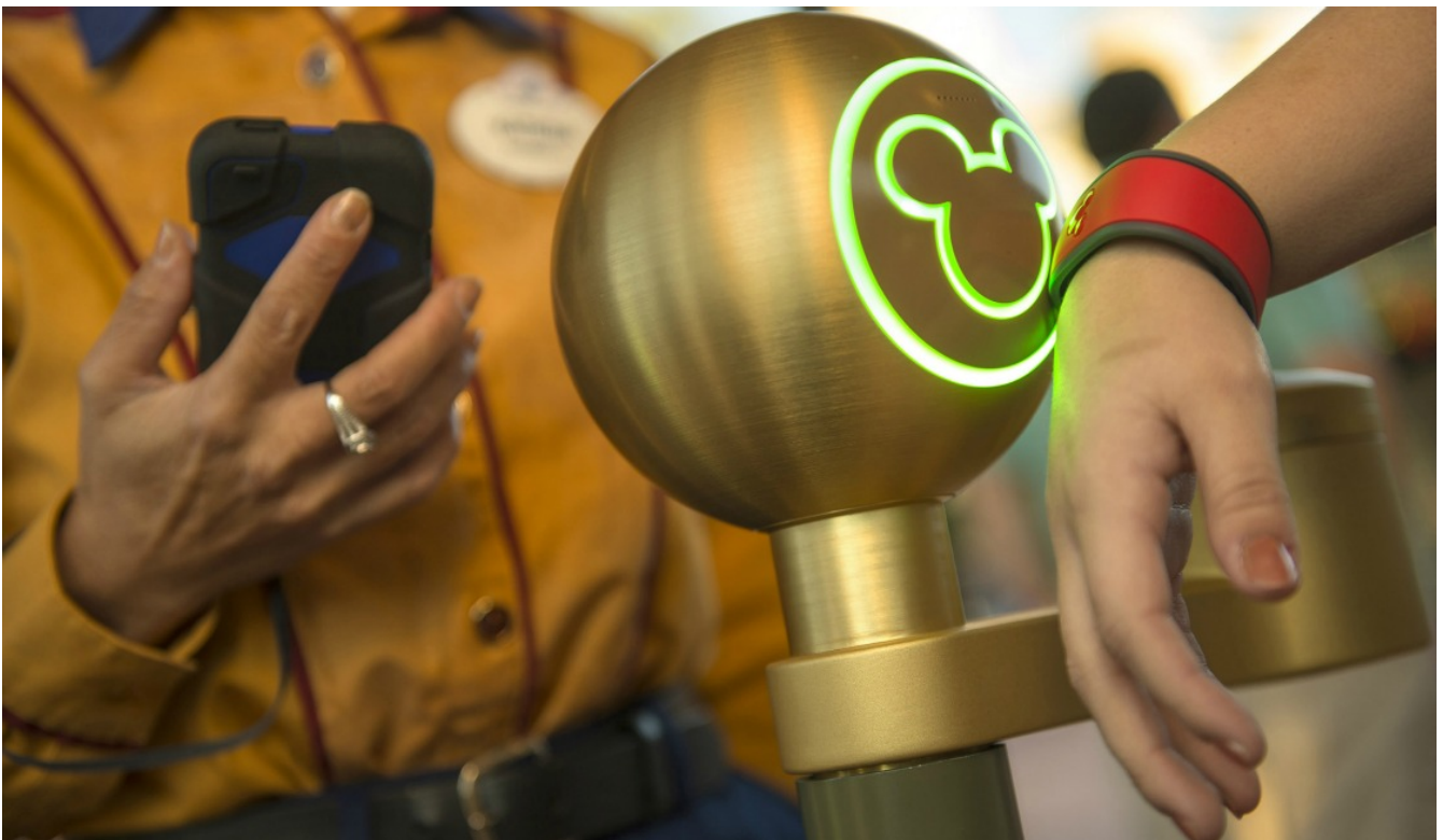
Figure 3. The "MagicBand" by Disney which acts as an entrance ticket and e-wallet
